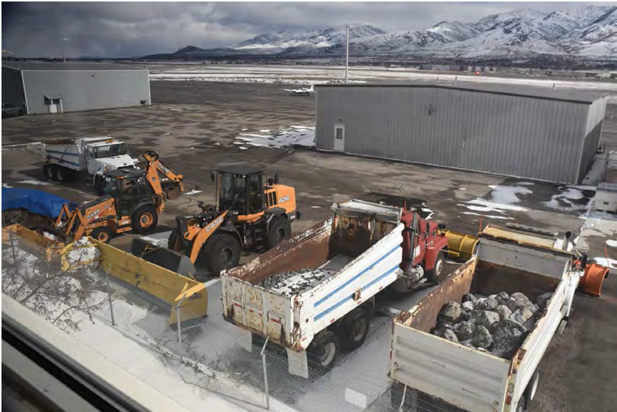
Figure 4: The LCCA snow control equipment is old, in poor condition, and insufficient for modern Part 139 operations. From left to right: the old snow-eater, two runway plows, and two highway style plows.
