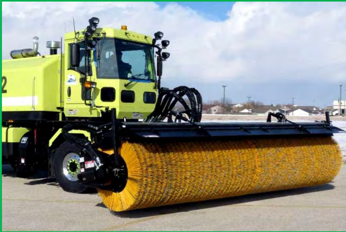
A modern Snow Broom Cleans Runways, Avoids Leaving a Thin Layer of Ice on the Pavement
