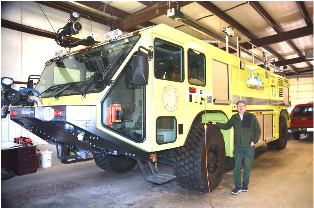
Figure 8: Airport Authority Chairman John Kerr checks out the LCCA "Stryker" fire fighting and rescue engine. Despite only having 20 miles on the odometer, this machine will need to be replaced within three years or the airport will lose Part 139 status. Another concern is the tires have a shelf-life, these have expired and need to be replaced at a cost of $8,000 per tire.
