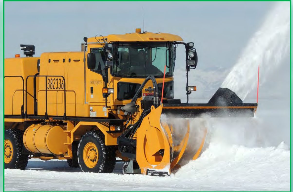
A Snow Eater Allows the Operator to Throw the Snow without Covering Landing Lights and Signs
